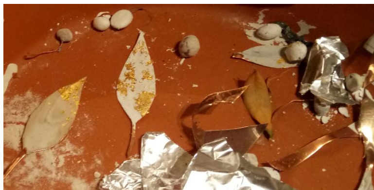
Figure 12. Leaves with coatings of calcite (left), kaolinite and a mixture of fuller's earth and calcite on a copper base.
