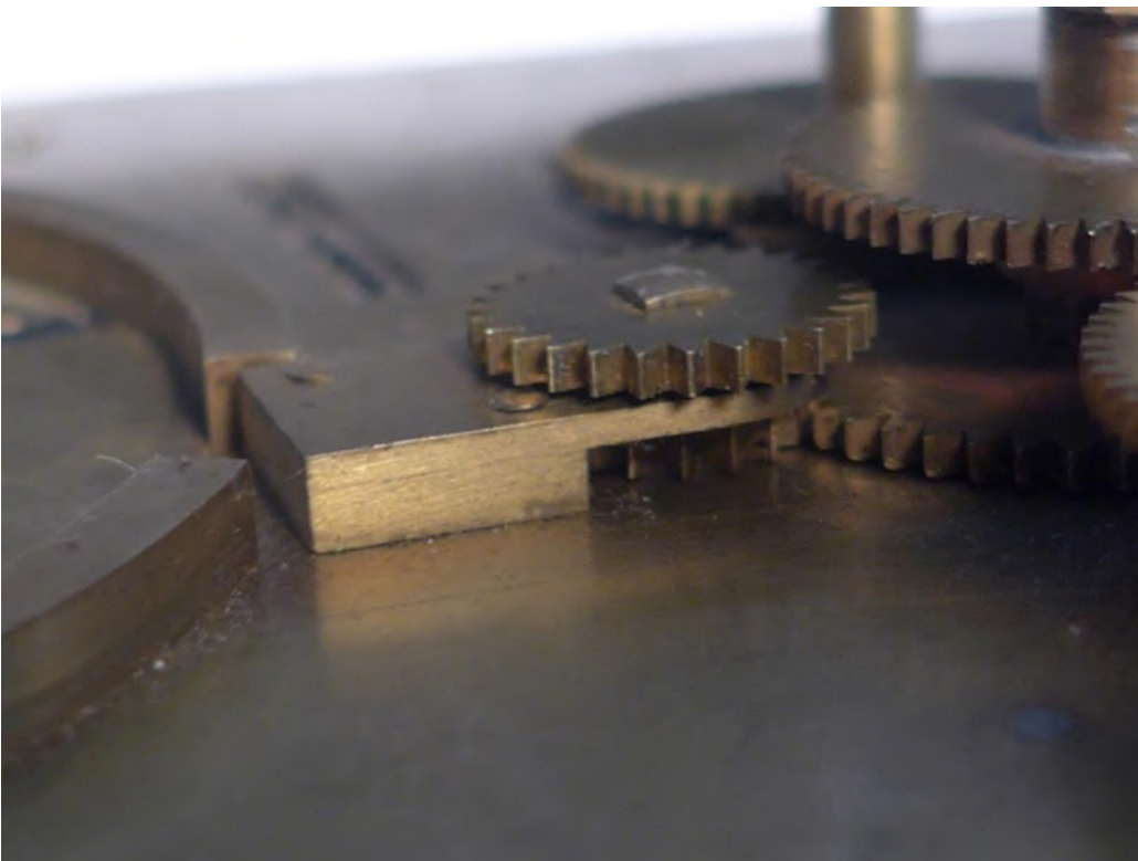
Figure 6. Antikythera Mechanism, detail showing cock on axis M, with wheel M2 seen below and wheel M3 above. Parts of a model of the Antikythera Mechanism built 2001/2, wheel M3 added 2006. © M.T. Wright.
