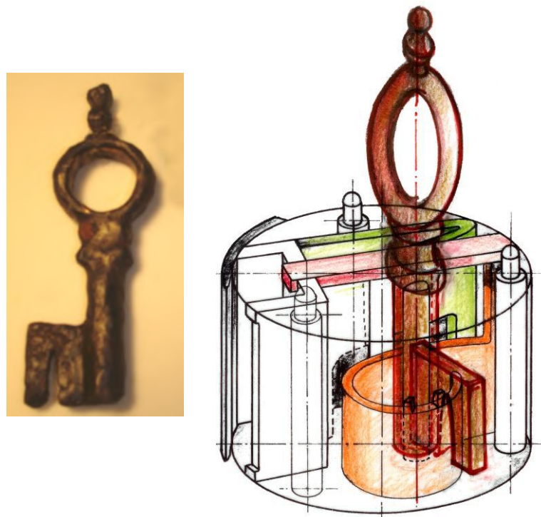
Figure 14: The key and its position in the spiral cam of the mechanism
