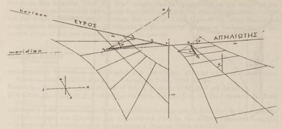
FIG.1 Partial view of the sundials at the South-east and East-face showing different cardinal parameters.
